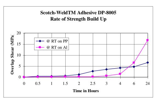
The above rate of strength build up was collected on 25mm\*100mm Aluminium and PP samples overlapped 12.5mm allowed to cure at 24°C and tested at a rate of 10mm/mn in overlap shear mode at 24°C.
